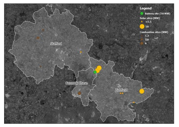
Figure 7—1 Existing or approved renewable sites in the LAEP boundary. Data is from the UK Renewable Planning database with background imagery from Google Satellite.
