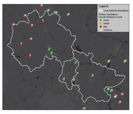
Figure 8—2 RAG analysis to provide an indication of available capacity at the primary substations in the LAEP area. Basemap from ESRI with substation data provided by WPD.
