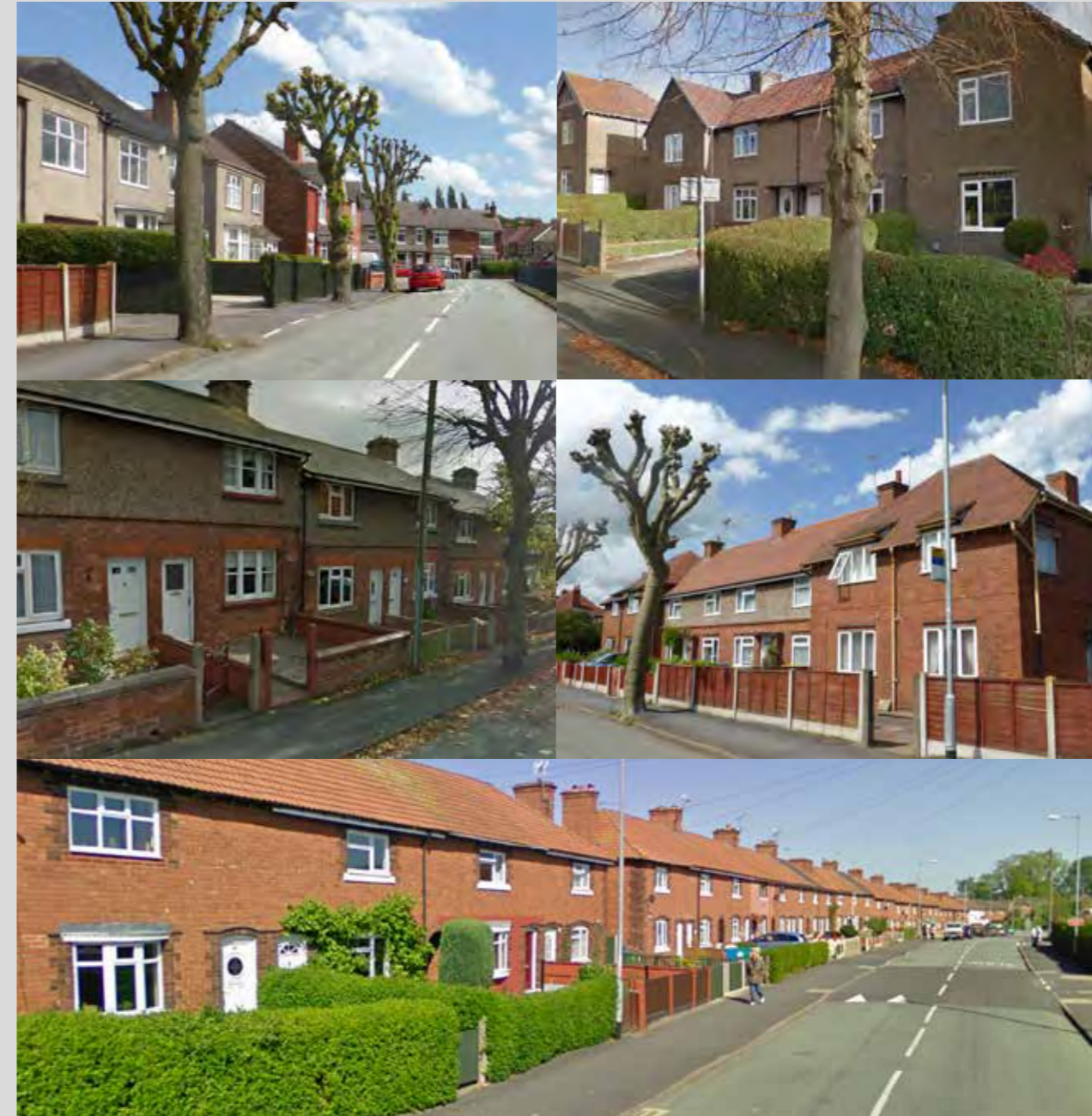
Post war terraced houses . 4 or 8 unit terraces, 8 house terraces have ginnels to rear gardens. Predominantly red brick with some painted rough cast render. Some houses with pebble dashed first floor. Roofs are a mix of slate and red tile. Front gardens vary between 3 to 10 metres.
