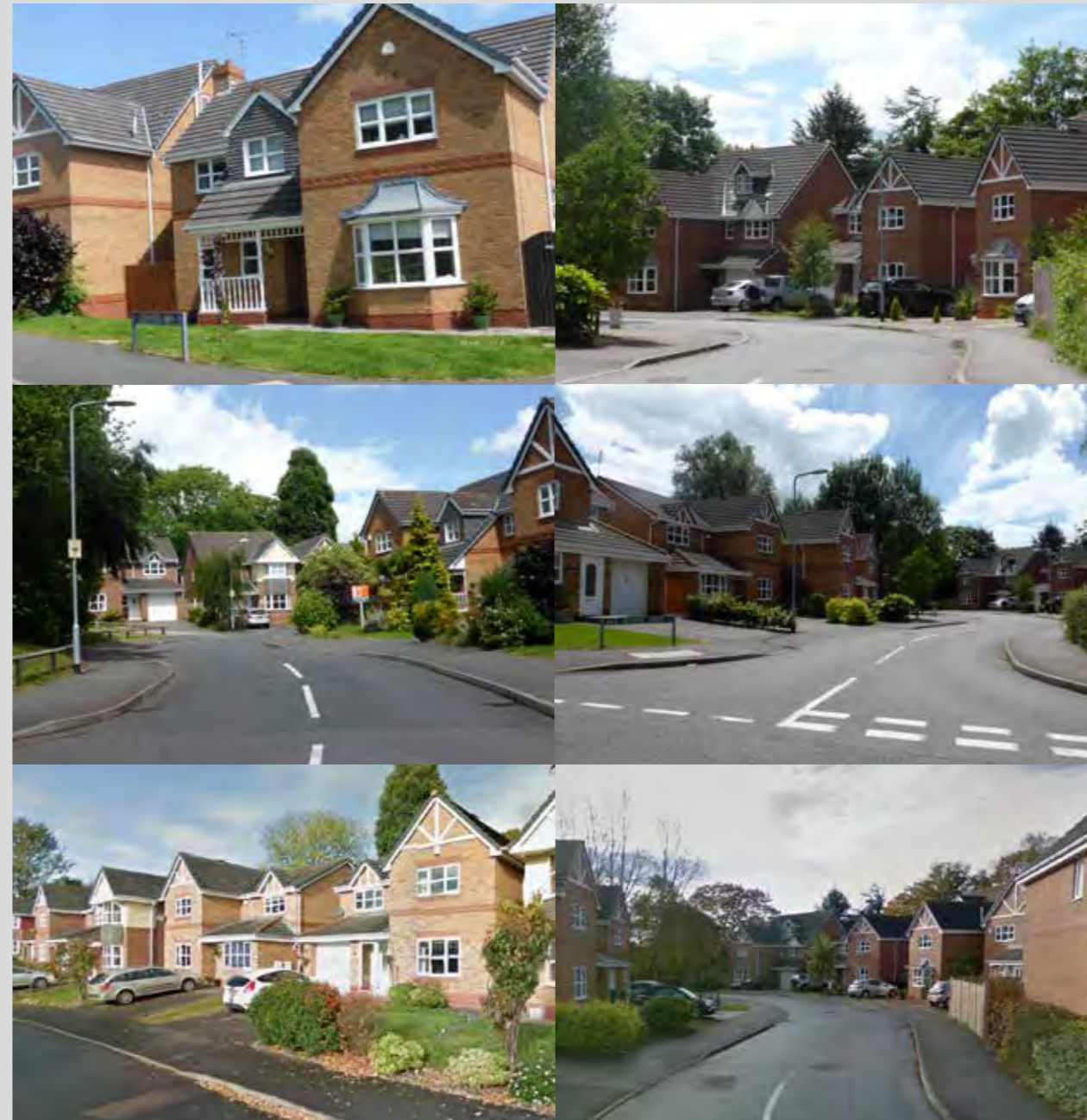
Recent development detached properties complex roof forms with front and end gables small gables above windows, multi colour brick with red brick detailing, grey tiled roofs 3 to 5 metre front gardens, on plot parking in detached or integral garages
