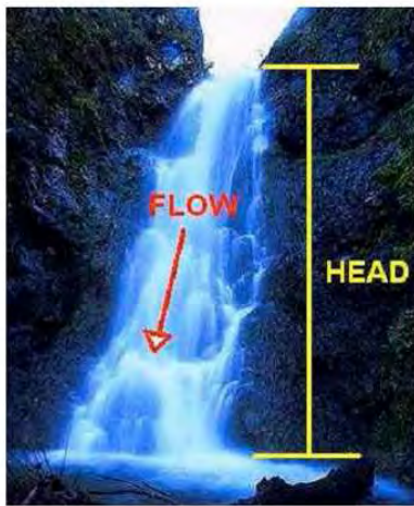
Figure 57: Hydropower – Head and Flow (Source: British Hydropower Association – UK Mini Hydro Guide)
